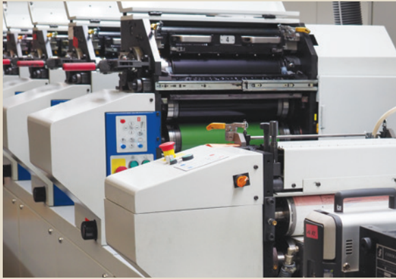
A Zahara NWL plate is seen mounted on 1.2.3. Etiketten's Codimag narrow web UV waterless offset press.
